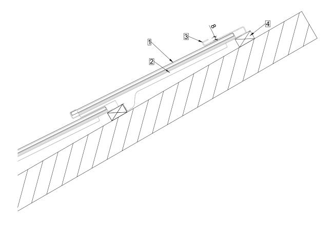
Modules that are not sufficiently secured with a MATCH Slate hook above them can be secured against wind suction with the MATCH Slate ridge hook.
