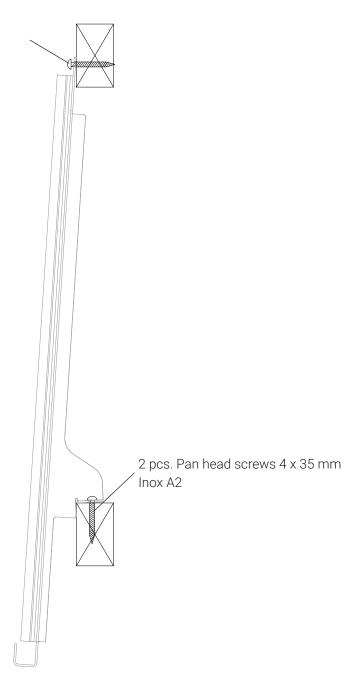
The MATCH hooks are screwed to the roof battens with 2 screws each. The screw at the top can be attached additionally, it is recommended especially in the top rows and in the edge areas. We recommend screwing the roof battens as well as the counterbattens. The static of the entire roof structure is the responsibility of the contractor.
