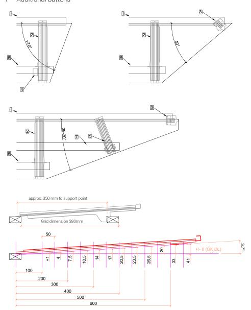
The layout of the match slate hooks must be adapted to the module angle.
