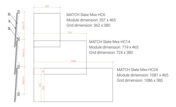
The grid dimension of the MATCH Slate modules is 380 mm in height, it can be adjusted by  $\pm 10$  mm. The grid dimension in width can be extended up to 10 mm.
