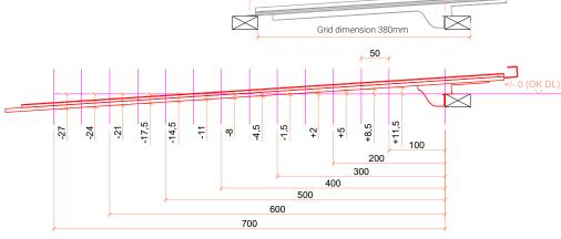
The layout of the match slate hooks must be adapted to the module angle.
