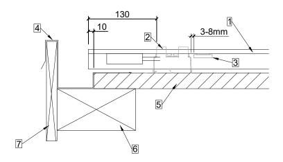
The MATCH adhesive fixation is applied during module assembly. Adhesive surface must be cleaned beforehand.
