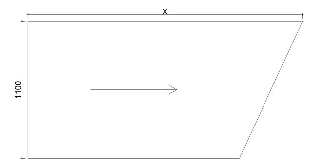
LEVEL Aluminium composite modules have a black matt coating. This coating is protected with a foil. Lay the modules so that the arrows on the foil point from left to right when looking at the roof from the front.
